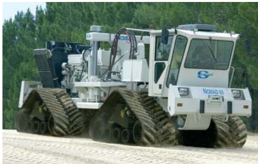
Off-road seismic vibrator Nomad 65T
